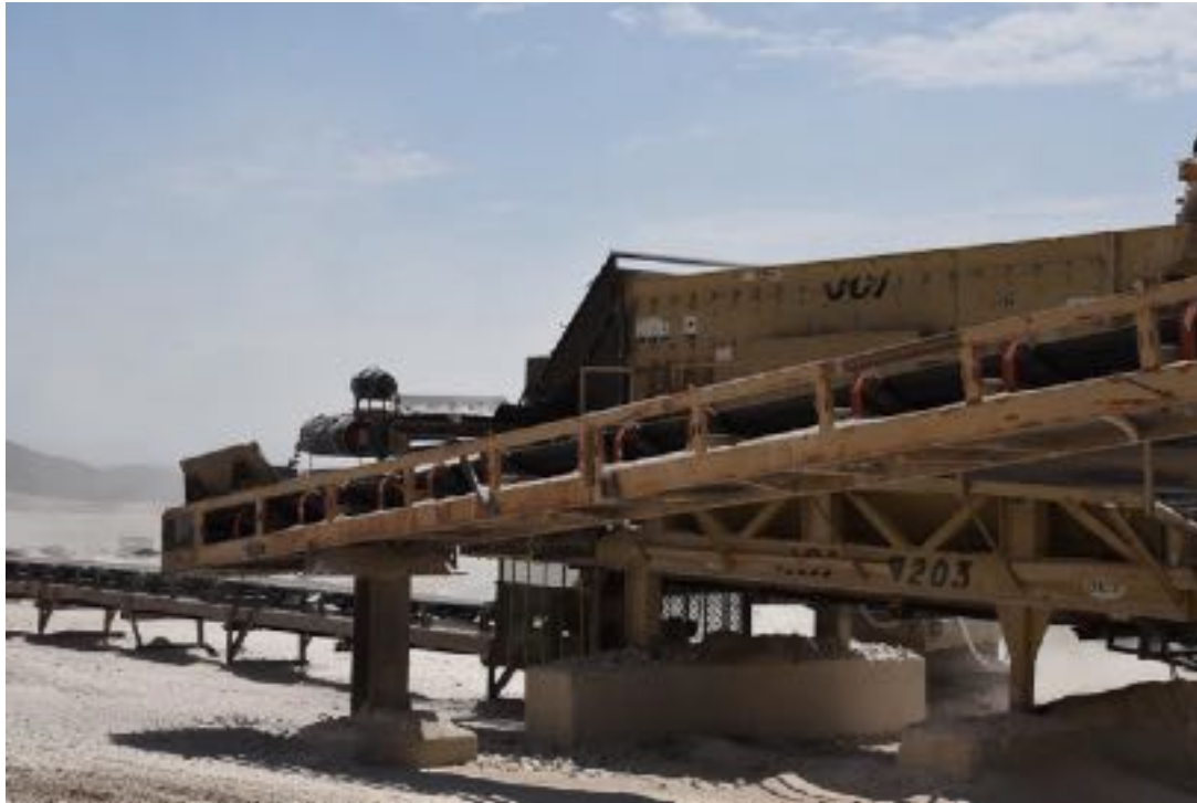
Figure 1.09a - Conveyor system returning over-sized fragments to crusher. Figure 1.09b - Crushed rock that meets ballast size specification are transported by a second conveyor and then deposited in pile at end of conveyor system. Photos by BK Darling.
