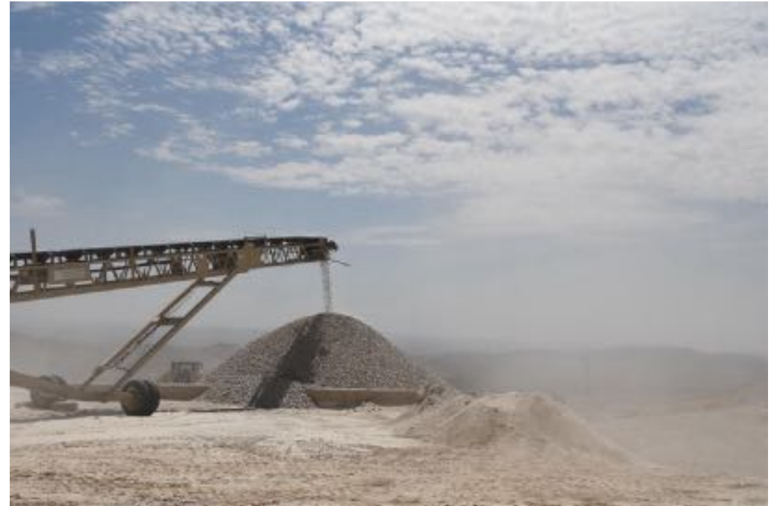
Figure 1.09a - Conveyor system returning over-sized fragments to crusher. Figure 1.09b - Crushed rock that meets ballast size specification are transported by a second conveyor and then deposited in pile at end of conveyor system. Photos by BK Darling.
